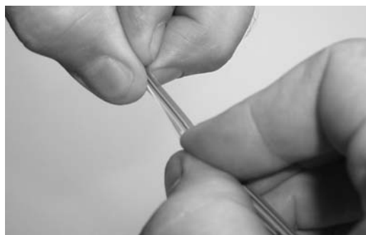
Figure 2.1: Folding the 24 Fiber Ribbon
