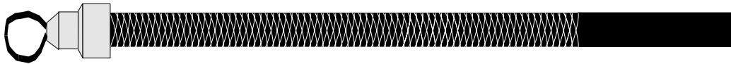
Figure 2: Completed Setup on FusionLink™ or UniLink™ cables with Grip Applied Over Cable Jacket.
