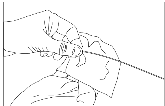
Wiping excess thixotropic gel from the fiber(s) or ribbon(s)
