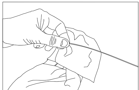
(Figure 3.3.b) Wipe excess thixotropic gel from the fibers or ribbons
