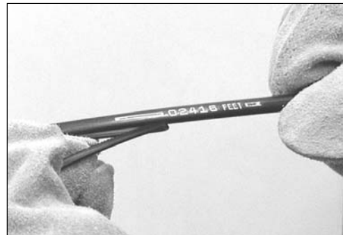
Fig. 4 Pulling off Toning Wire
